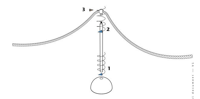
If you want the components to be locked, use the threadlocker sold on www.e-spheria.com
