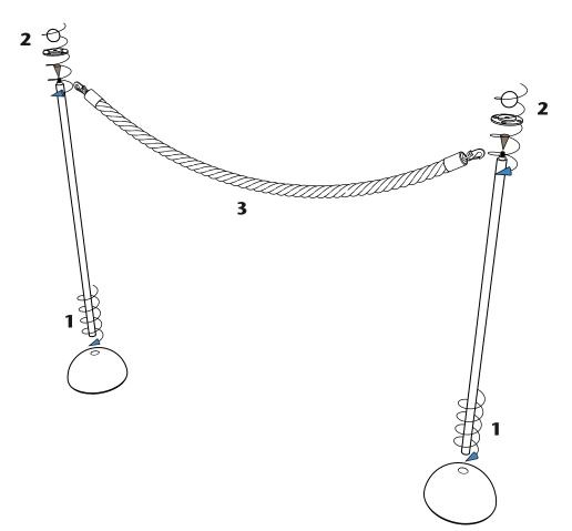
If you want the components to be locked, use the threadlocker sold on www.e-spheria.com
